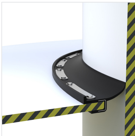
DAFA RotaSeal® Straight Profile sealing for rotating parts. Mechanically fastened on the horizontal flange on the nacelle bottom cover.
