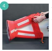
Wrap the tip protector very tightly by pulling hard using both hands.
