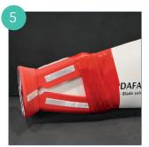
After winding 5 times around, cut off the roll of tape. Ensure the last layer only touches the blade.
